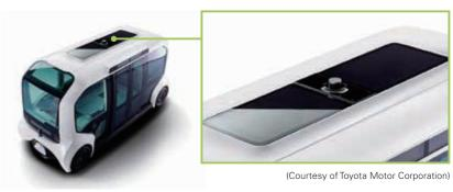
(Photo 2) Kaneka's solar cell installed in the roof glass of Toyota's low speed automatic driving EV "e-Palette
