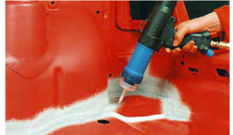
Kaneka MS Polymer used as automotive repairing agents
