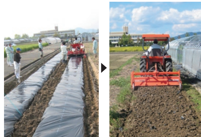
Testing the usage of agricultural multi-film. After five months on the ground (left), the film has decomposed sufficiently to allow a farmer to plough it into the soil (right)
