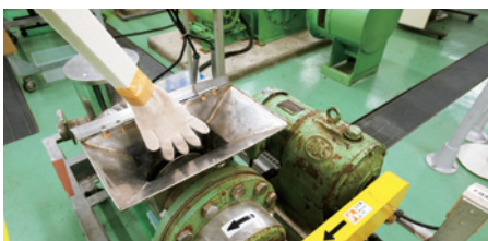
Conveying accident risks more realistically by using a stick modeled as an arm wearing a work glove
