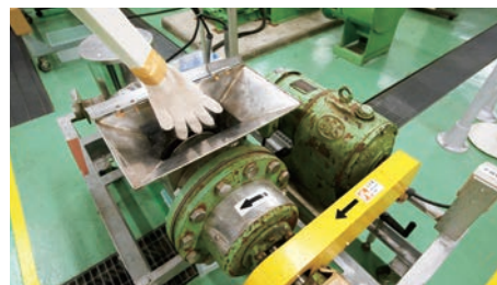
Conveying accident risks more realistically by using a stick modeled as an arm wearing a work glove
