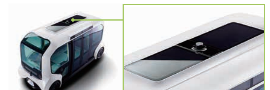
(Photo 2) Kaneka's solar cell installed in the roof glass of Toyota's low speed automatic driving EV "e-Palette" (Courtesy of Toyota Motor Corporation)
