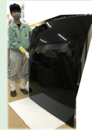
Solar roof (prototype) heterojunction back-contact crystalline silicon solar cell
