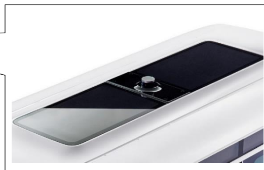
Kaneka's photovoltaic modules installed in the roof glass
